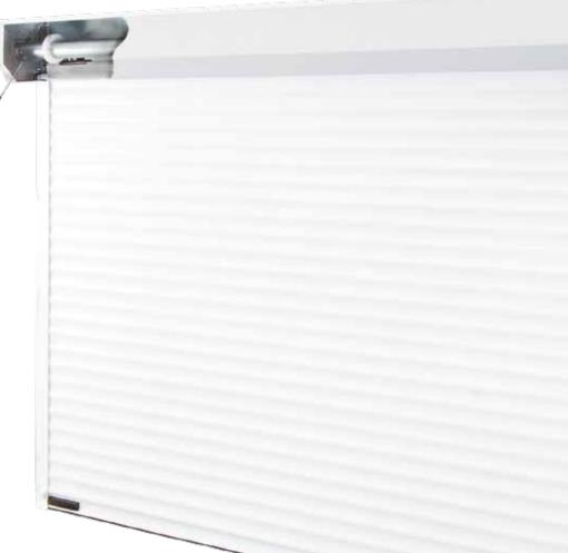
Gliderol Insulated Roller Doors take up very little space inside your garage. The standard configuration, using 77mm foam filled lath, requires 300mm of headroom and is supplied with 70 or 90mm guides depending on specification. The compact version, using 55mm foam filled lath, requires only 205mm of headroom and is supplied with 65mm guides.
